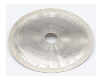
These thin rim sintered diamond sawblades last longer than notched blades. The diamonds (325#/400#) are secured into a metal bond that extends the full depth of the rim. Diamonds are continuously exposed as the edge of the blade wears away cut after cut. They offer a long life and clean, thin cuts. Click to enlarge the image to see a close-up of the diamonds secured in the rim.
