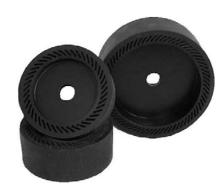
Angled expansion slots through the heavy rubber rim allow the drum to expand when rotated; thereby locking the belt in place.
