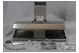
This machine made by Our Company in an all 304 grade stainless steel construction, 3/4" stainless steel shafts and ball bearings. It also has a rear mounting plate and motor hood, We also can supply a adjustable drip water system with 6
