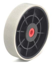
These Wheels are made with a cross hatch pattern that allows for fast grinding. The new textured design also prevents chipping of Lapidary and glasswork. All wheel arbor is 1" comes with reducing bushing in 3/4", 5/8", and 1/2".
